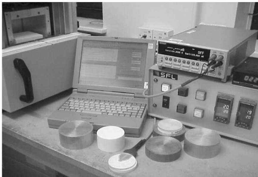
Fig. 1. TPS sensor and samples with computer, PSU, voltmeter, and chamber for the temperature range -60 to 400^{\circ}\text{C} .
